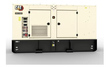
Maximum Rating 310 kVA Minimum Rating 310 kVA **Emissions** EU Stage V 400 V Voltage 50 Hz Frequency Height 2.277 mm Length 4.085 mm Width 1.514 mm Dry Weight 4.103 kg
