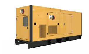
Rated Speed 1500/min Minimum Rating 780 kVA Frequency 50Hz 400 V Voltage Engine Model C18 Dry Weight - Genset 4.322 kg Height 2.155 mm Length 3.900 mm Width 1.461 mm Maximum Rating 780 kVA
