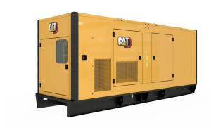
Rated Speed 1500/min Minimum Rating 715 kVA Maximum Rating 715 kVA Frequency 50Hz Voltage 400 V **Engine Model** C18 Dry Weight - Genset 4.372 kg Height 2.155 mm Length 3.900 mm Width 1.461 mm
