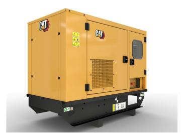
Minimum Rating 13,5 kVA Rated Speed 1500 rpm Frequency 50 Hz 400 V Voltage Engine Model C1.5 Dry Weight - Genset 384 kg Height - Maximum 1.054 mm Length - Maximum 1.400 mm Width - Maximum 620 mm Maximum Rating 13,5 kVA
