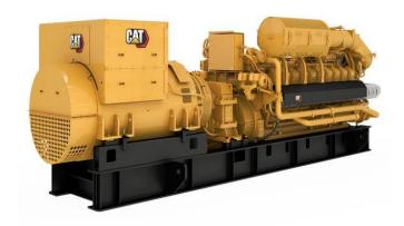
Maximum Electrical Efficiency 45,2% Displacement 97,6 I Bore 170 mm Stroke 215 mm Compression Ratio 12,1:1 Fuel Type Natural Gas Maximum Power 2.526 kW Rated Speed 1500 rpm Minimum Power 1.247 kW
