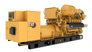
Fuel Type **Natural Gas** Displacement 58,5 I Bore 170 mm Stroke 215 mm Maximum Electrical Efficiency 44,8% Maximum Power 1.516 kW **Compression Ratio** 12,1:1 Rated Speed 1500 rpm Minimum Power 749 kW
