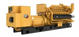
Maximum Continuous Rating 2022 ekW Fuel Type Natural Gas Maximum Electrical Efficiency 41.50% Maximum Standby Rating 2.022 Frequency 50 **RPM** 1.500 **Engine Model** G3520E 86 I Displacement Aspiration TA Bore 170 mm Stroke 190 mm Length 6.893 mm Width 2.001 mm Height 2.727 mm 17.826 kg Dry Weight - Genset Fuel System Natural Gas **Compression Ratio** 11,9 Minimum Rating 2.022 kVA Maximum Rating 2.022 kVA Rated Speed 1500 rpm
