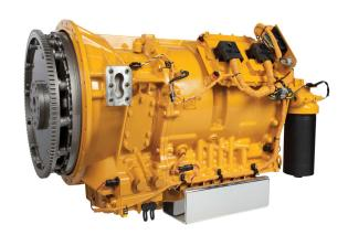
Gross Peak Input Torque 2.700 N·m Rated Input Speed 2.100 r/min Maximum Turbine Torque 2.700 N·m Minimum Input Speed 600 r/min **Electrical System** 12 V Gear Type Planetary Spur 8F/1R Gears 1F Gear Ratio 5,73 2F Gear Ratio 3,57 3F Gear Ratio 2,72 4F Gear Ratio 1,95 5F Gear Ratio 1,43 6F Gear Ratio 1 7F Gear Ratio 0,74 8F Gear Ratio 0,63
