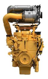
Power Range Maximum Power Minimum Power Emissions Rated Speed Bore Stroke Displacement Compression Ratio Dry Weight Length Width Height 340-430 kW (456-576 bhp) 430 kW 340 kW EU Stage V, U.S. EPA Tier 4 Final 1800 - 2000 rpm 130 mm 157 mm 12,5 l 15,8:1 1.125 kg 1.274 mm 994 mm 1.134 mm
