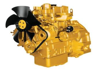
Maximum Power 13,3 kW Maximum Torque 44 Nm @ 1600 rpm Rated Speed 2200-3600 rpm Minimum Power 8,8 kW Emissions U.S. EPA Tier 4 Final, EU Stage V Engine Configuration In-Line 3 Bore 67 mm 72 mm Stroke Displacement 0,76 l **Compression Ratio** 23.5:1 Naturally Aspirated (NA) Aspiration **Combustion System** Indirect Injection Rotation from Flywheel End Counterclockwise 480 mm Length Width 371 mm Height 528 mm Weight - Net Dry - Basic Operating Engine 71 kg Without Optional Attachments
