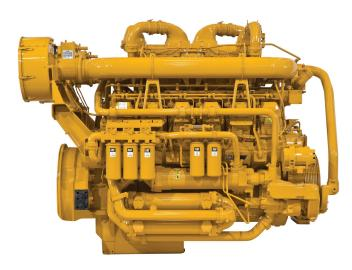
Maximum Power 746 kW 4.263 Nm @ 1600 rpm Maximum Torque Rated Speed 1200-1800 rpm **Minimum Power** 507 kW Emissions Non-Certified Engine Configuration V-8, 4-Stroke-Cycle Diesel Bore 170 mm 190 mm Stroke Displacement 34,5 I **Compression Ratio** 13.0:1 **Turbocharged Aftercooled** Aspiration Rotation from Flywheel End Counterclockwise Aftertreatment Length 2.136 mm Width 1.703 mm Height 1.720 mm Weight - Net Dry - Basic Operating Engine 4.309 kg Without Optional Attachments
