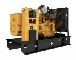
Minimum Rating 330 kVA Rated Speed 1500/min Maximum Rating 330 kVA Frequency 50 Hz Voltage 400 V Dry Weight - Genset 3.280 kg Height - Maximum 1.760 mm Length - Maximum 3.300 mm Width - Maximum 1.110 mm **Engine Model** C9
