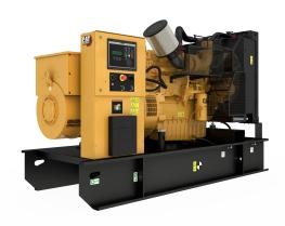
Minimum Rating 300 kVA **Power Range** 1500/min Frequency 50 Hz 400 V Voltage **Engine Model** C9 Height - Maximum 1.760 mm Length - Maximum 3.300 mm Width - Maximum 1.100 mm Dry Weight - Genset 2.483 kg
