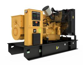
Minimum Rating 250 kVA Rated Speed 1500/min Maximum Rating 250 kVA Frequency 50 Hz Voltage 400 V **Engine Model** C9 Height - Maximum 1.718 mm Length - Maximum 2.662 mm Width - Maximum 1.030 mm
