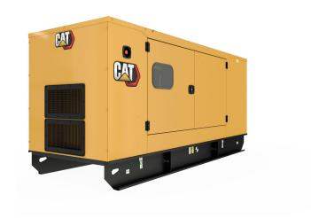
Minimum Rating 165 kVA Rated Speed 1500/min Maximum Rating 165 kVA Frequency 50 Hz Voltage 400 V **Engine Model** C7.1 Dry Weight - Genset 1.735 kg Height - Maximum 1.528 mm Length - Maximum 2.500 mm Width - Maximum 1.120 mm
