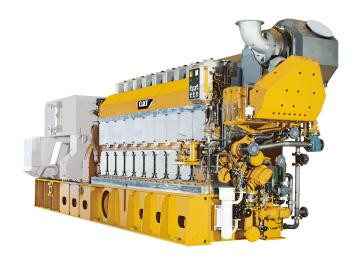
Minimum Rating 3.880 ekW 3.880 ekW Maximum Rating **Emissions** IMO Tier II 309 I Displacement **Generator Set Control** Electronic Weight 93.000 kg Bore 320 mm 480 mm Stroke
