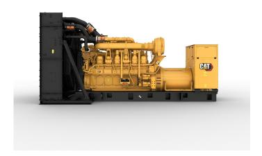
Minimum Rating 1.600 kVA Maximum Rating 2.525 kVA Rated Speed 1500/min Voltage 400 V Frequency 50 Hz Width 2.091 mm Length 5.523 mm Height 2.332 mm Dry Weight - Genset 14.520 kg **Engine Model** 3.512
