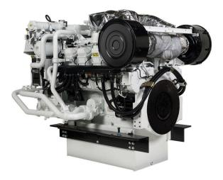
Power Range 775-1100 bhp (578-820 bkW) Speed Range 1200-1600 rpm Emissions IMO II, EU IW Aspiration TTA Bore 170 mm Stroke 190 mm Displacement 34,5 I Rotation from Flywheel End Counterclockwise or Clockwise Configuration Vee 8, 4-Stroke-Cycle Diesel Minimum Dry Weight 4.960 kg Length 2.117 mm Height 1.829 mm Width 1.703 mm **Minimum Power** 578 kW Maximum Power 820 kW IMO II, EU IW Emissions
