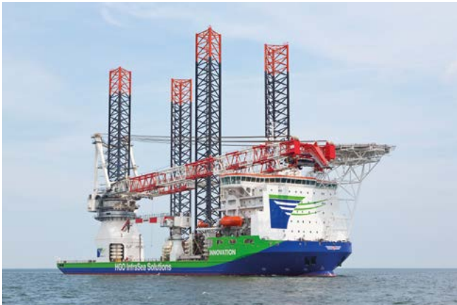
Offshore 6x MaK 9 M 32 C, 1x MaK 9 M 20 C, 1x CAT C32
