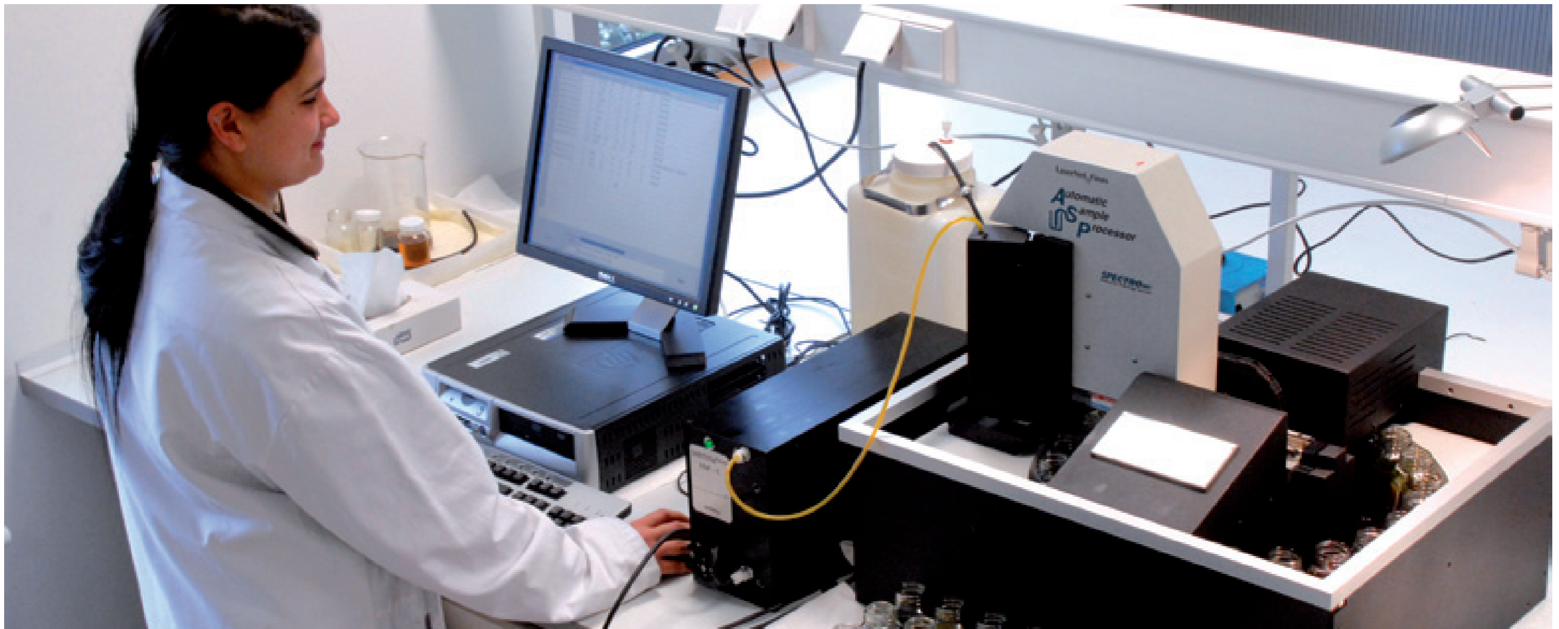
Particle counts to determine oil purity
